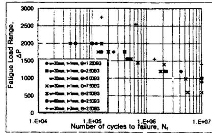
**Fig. 6**  $\Delta P-N_f$  relation of spot-welded lap joints
