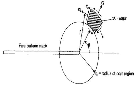
Fig. 2 2-dimensional core region surrounding the crack tip
