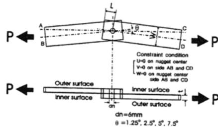
**Fig. 3** Configuration of IB type spot-welded lap joint
