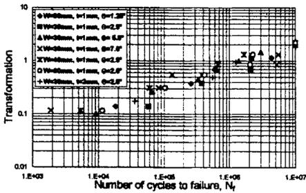
Fig. 9 Relationship between transformation function and failure life
