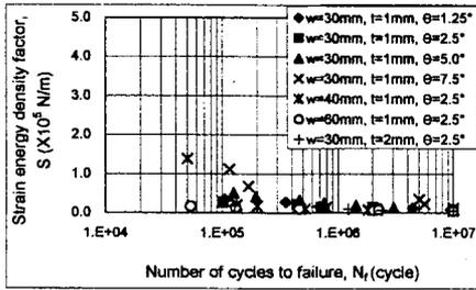
Fig. 7  $S-N_f$  relation of spot-welded lap joints
