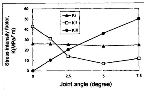
Fig. 5 Variation of stress intensity factors against joint angle. ( $P=9.81$ MPa)
