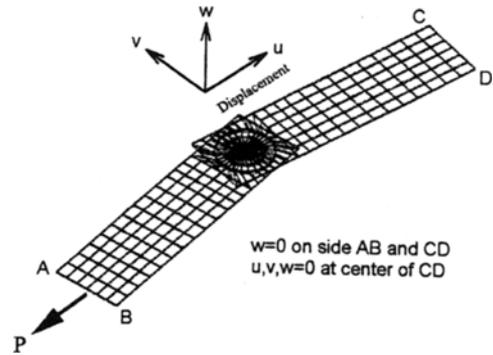
**Fig. 4** The 3-dimensional finite element analysis model of IB type spot-welded lap joint
